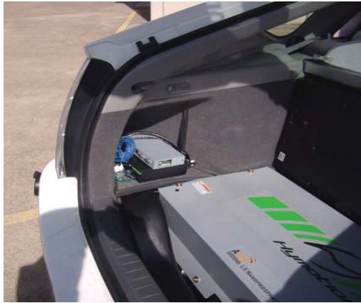
Figure 2. Sensors located throughout the PHEV connect to data logger and transmitter in the rear of the vehicle. The system enables Austin Energy engineers to monitor and record operating parameters in real time. The large L5 nano-phosphate lithium ion battery seen at the lower right of the photo is manufactured by A123 Systems of Watertown, Massachusetts.
