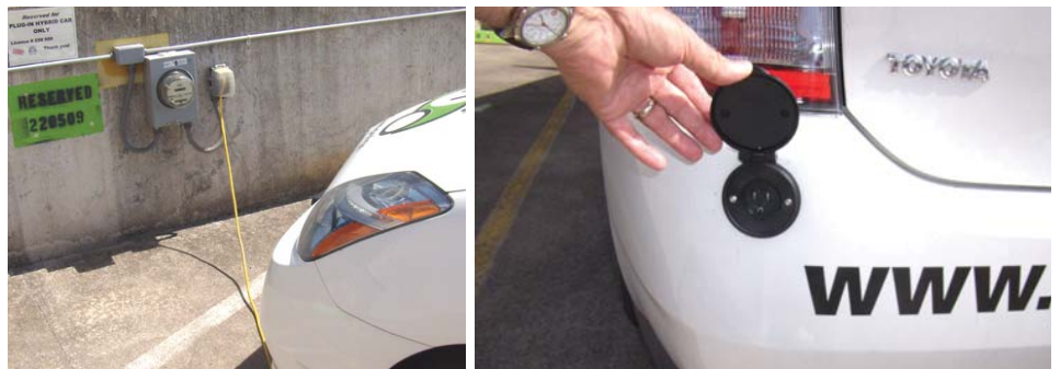
Figure 3. Austin Energy installed a 120-V charging station and meter on the roof of its parking garage to monitor PHEV energy consumption (left). Note that charging requires only a standard AWG 12 extension cord, which is inserted in a receptacle mounted in the PHEV's rear bumper (right). Charging at 120-V takes about four hours, or about double the time needed with 240 V power.
