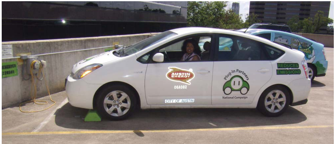
One of Austin Energy's two plug-in hybrid vehicles. The PHEVs are modified versions of the Toyota Prius and are fitted with lithium batteries large enough to extend their all-electric range to 20 miles. One of the utility's conventional Prius hybrids can be seen in the background.
