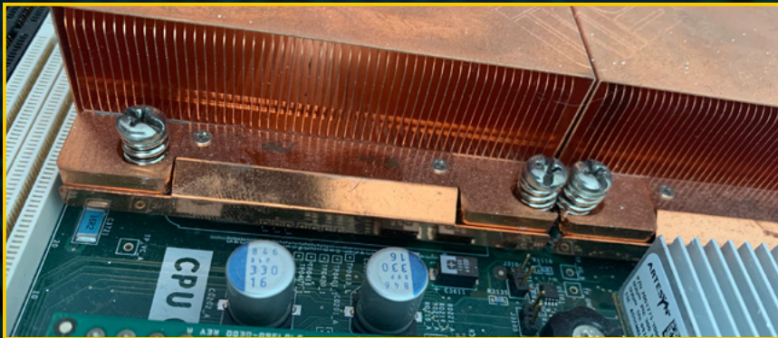
Figure 17: Covered Heat Sink
