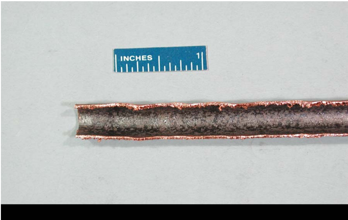
Figure 3. Close-up view of corrosion deposit on the inside of the bare copper sample after 52- weeks' exposure.
