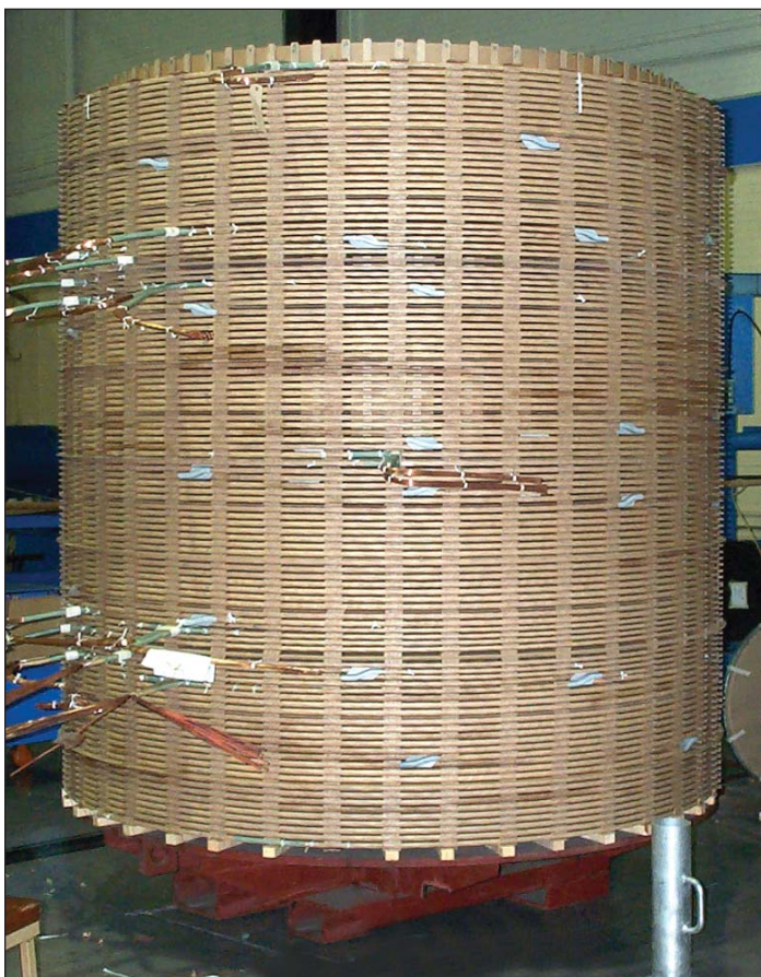
Figure 3. Finished coil for a large substation transformer showing paper insulation before oil impregnation. Thermal cycling can compress the insulation, a condition that can eventually lead to loose connections. Copper-wound transformers are much less prone to this effect than those wound in aluminum, one reason copper transformers are known for high reliability. (Photo courtesy Pennsylvania Transformer Technology, Inc.)
